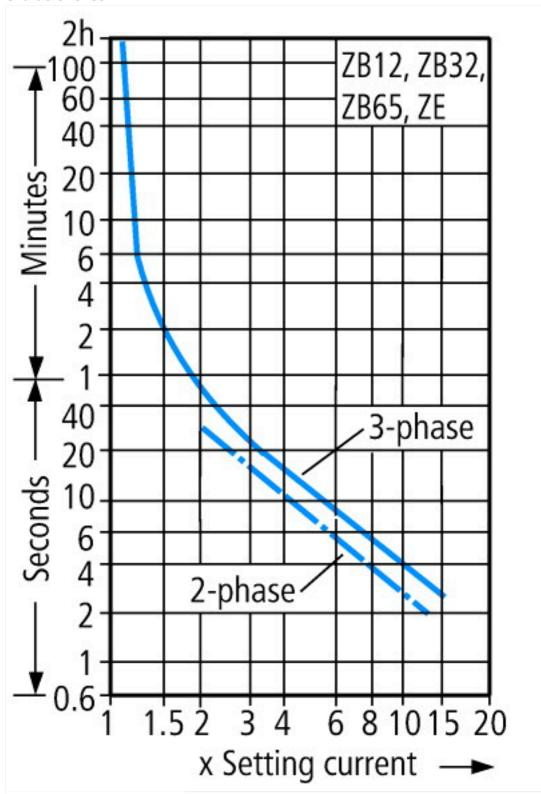
These tripping characteristics are mean values of the spread at 20 °C ambient temperature in a cold state. Tripping time depends on response current.
